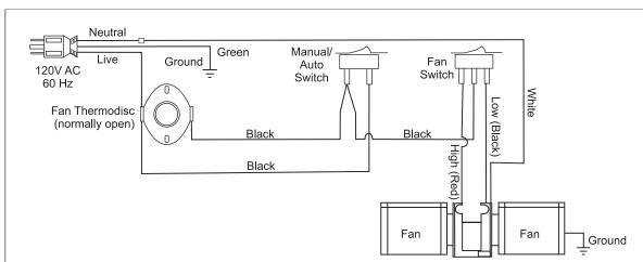
Blower/Fan Wiring Diagram
